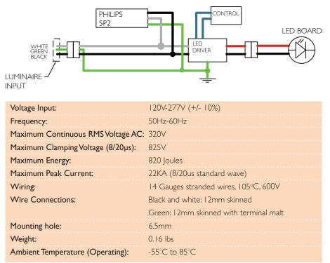
In order to protect the surrounding environment, this surge protection device must be enclosed in a luminaire that can contain flames and sparks, which may occur in case of malfunction, such as overvoltage power connection (ex:600V).
